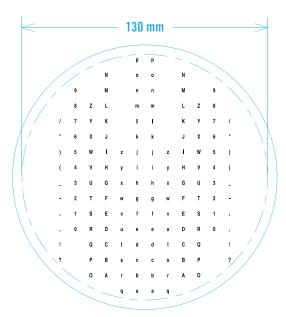
This is an example of a printing plate artwork layout for printing variable data on the SELECTA-150.
