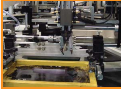
Servo driven printing station with pneumatic squeegee
