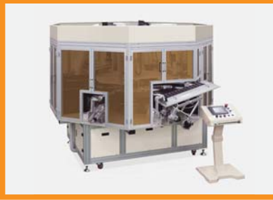
2 color TUBOY tube screen printing system shown
