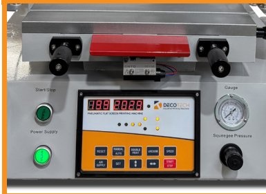
Close Up View of the Control Panel with Membrane Switches & LCD Display
