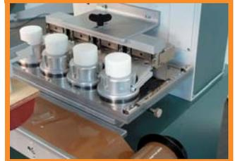
MSS-350 configured with open inkwell system
