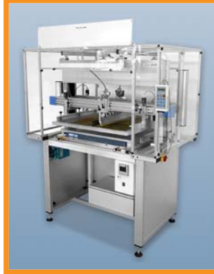
Set-up for printing heated cocoa butter onto chocolate transfer sheets
