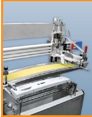
Shown with special tooling for printing arched appliance panels
