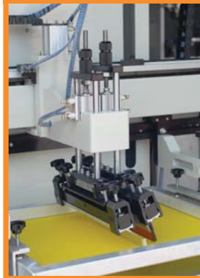
Squeegee & Floodbar Assembly with micro adjustability
