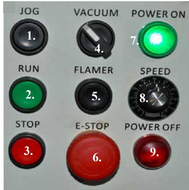
1. Pressing and releasing this button cycle the machine in steps.
