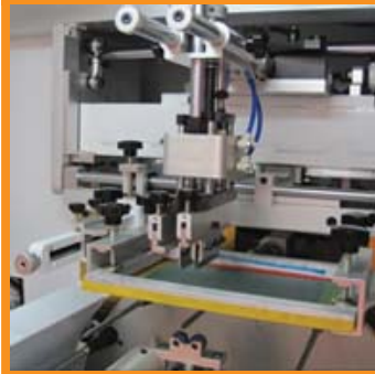
Close-up of print head with X/Y/R adjustment
